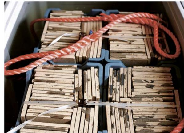
Cleaning of ceramic tiles in acid vinegar baths. Photo: Rotor.
